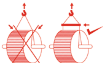
Lifting the cable drum by crane
