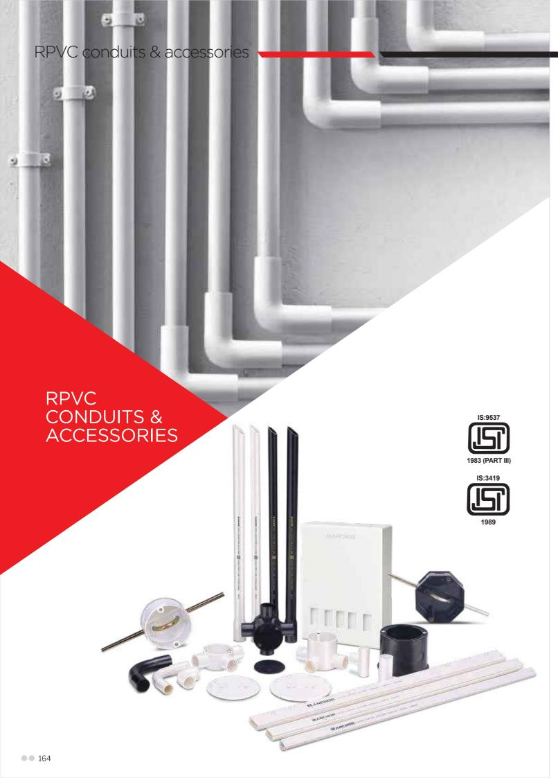
Anchor Rigid Conduit PVC Pipes and Accessories are manufactured from a specially formulated unplasticised ployvinyl chloride (UPVC) to meet stringent Indian standards. Our products are made of Extra Super High Impact material which make them safe to be use in harsh environments. The products are maufactured in accordance with IS:9537 (Part III) for PVC conduit pipes and IS:3419 for junction boxes.
