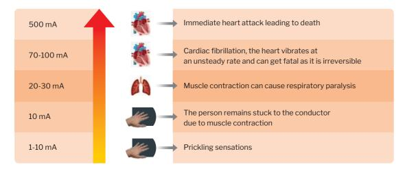
Electrocution should not be viewed in terms of "Current" alone, but in terms of "contact voltage". A person gets electrocuted by coming in contact with an object that has a different potential from his/her own. The difference in potential causes the current to flow through the body.
