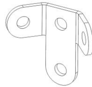
(2) Guy Wire Bracket (Used with UMH)
