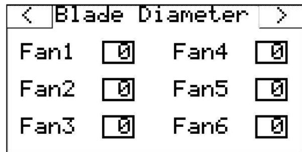
4. Optional: Set blade sizes (diameter) for each fan on the network (can be done through BACnet).
