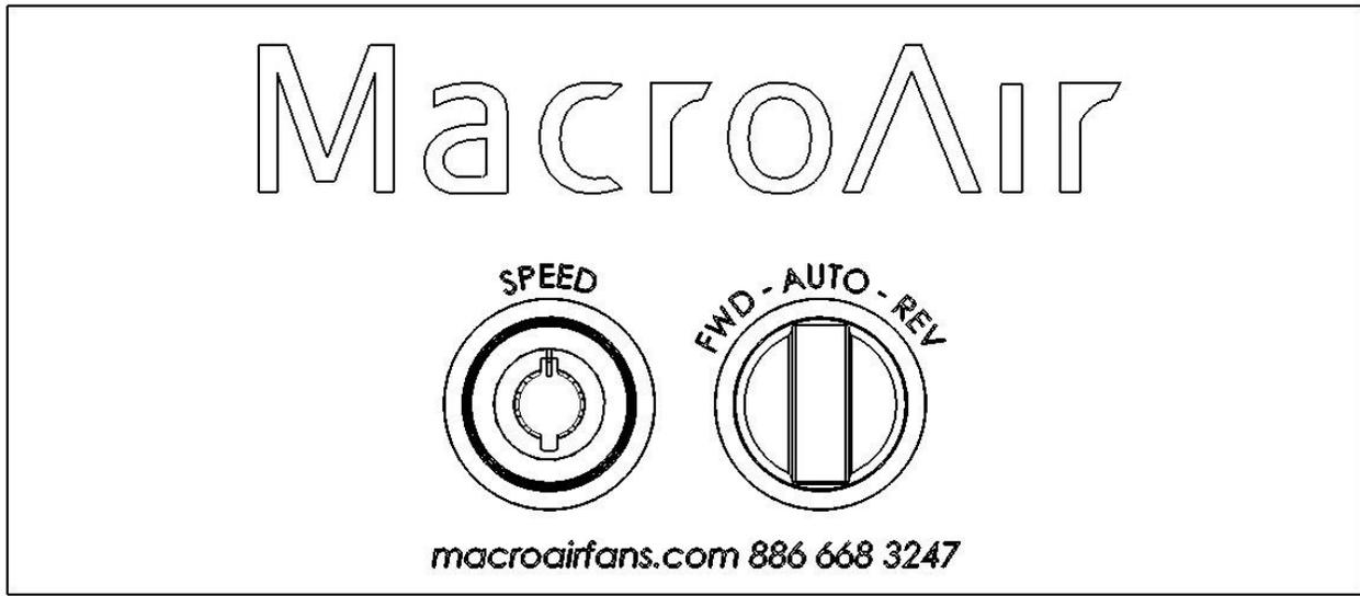
**OFF:** To turn off the fan set to FWD (forward) or REV (reverse) with a speed of 0. This will turn the fan off and prevent the BMS from running the fan.
