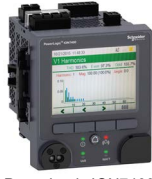
PowerLogic ION7400 with harmonics display.
